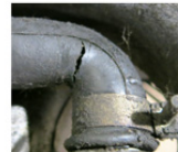
M110/M116/M117 Position of engine airduct rubber components underneath suction manifolds
